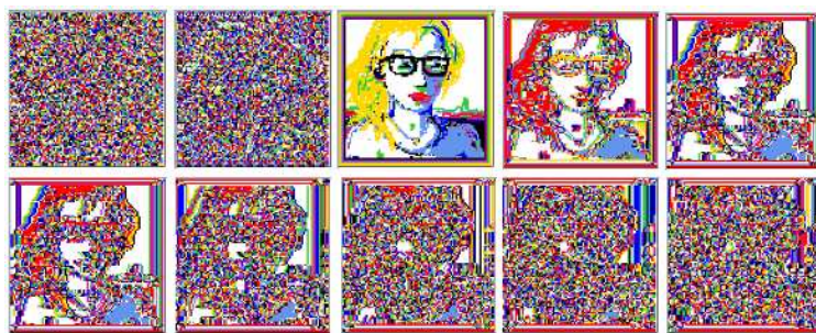
Fig. 9. To decrypt, starting from the encrypted state in Fig. 8 ( n=7744 , 88 \times 88 ), the CA with the same rule was run forward to recover the original image. This figure shows time steps -2 to +7.
