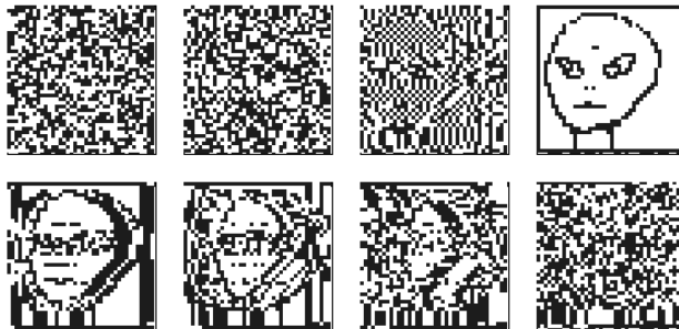
Fig. 7. To decrypt, starting from the encrypted state in Fig. 6 ( n=1600 , 40\times 40 ), the CA with the same rule was run forward by 20 time steps, the same number that was run backward, to recover the original image or bit-string. This figure shows time steps 17 to 25 to illustrate how the “alien” image was scrambled both before and after time step 20. This figure was taken from [8, 10].
